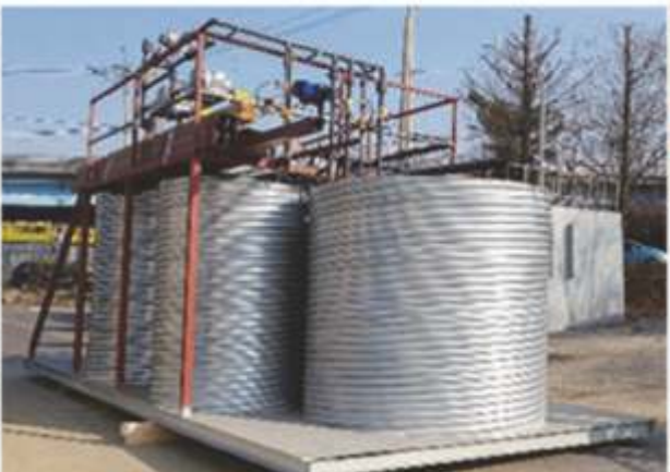
Package modularization (50m 3 /d HxWxL = 4x4x8m)
